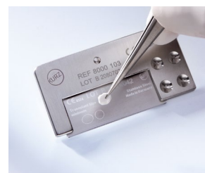
Blade with template for graft size determination
